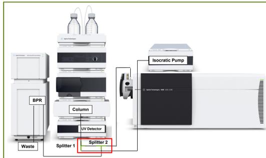
Figure 1) Configuration of the Agilent 1260 Infinity Analytical SFC Solution with the Agilent 6460 Triple Quadrupole LC/MS System. The column is directly connected to the splitter 1 in the splitter assembly (BPR = back pressure regulator, UV detector not used, Splitter Kit p/n: G4309-68715).
